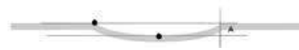
The deformation value is the height difference A between the two points shown
