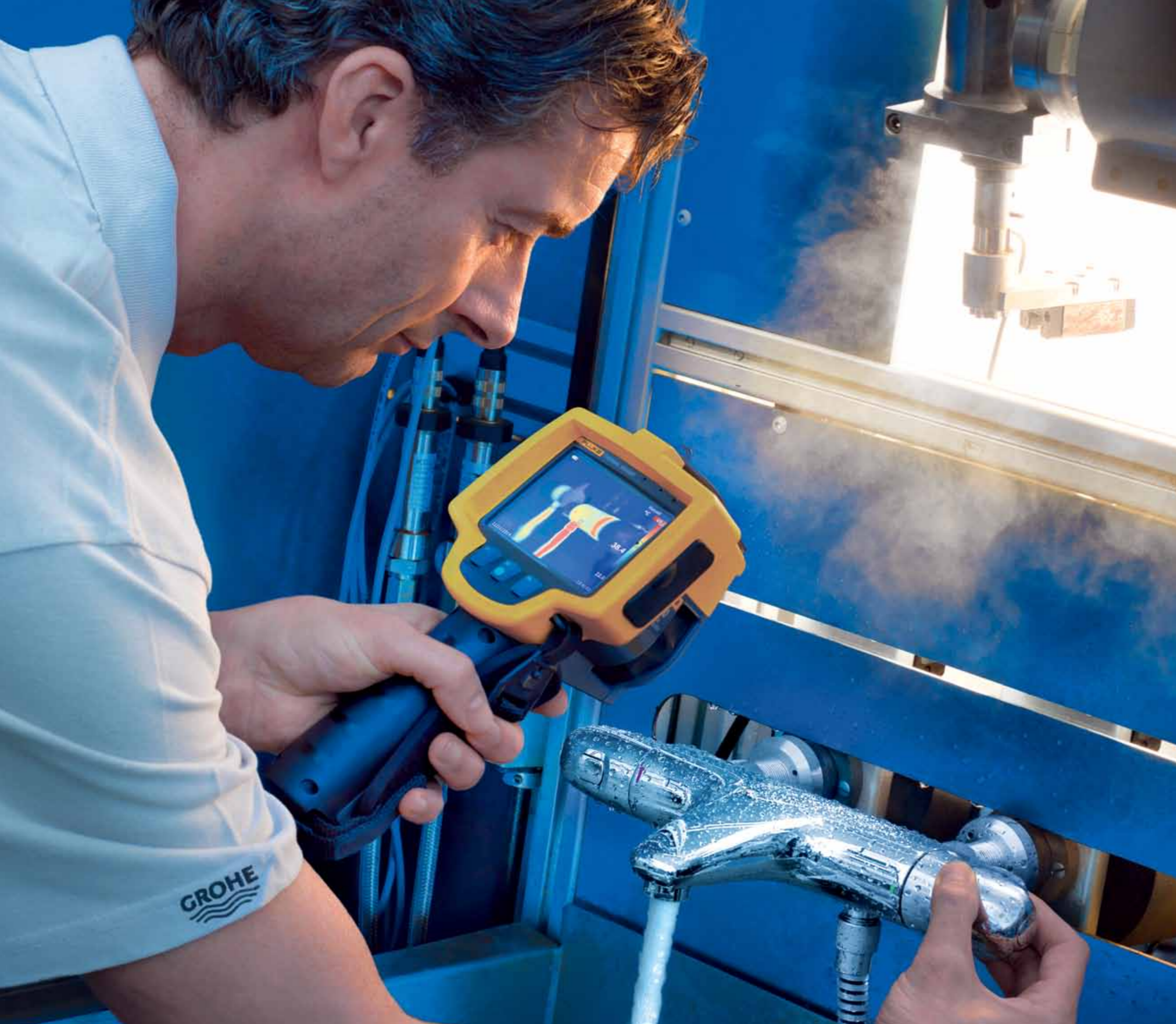
Ruurd van Leeuwen, Master of Technology, tests the built-in GROHE CoolTouch® technology, which ensures the shower surface stays at a safe temperature despite the flow of hot water.
