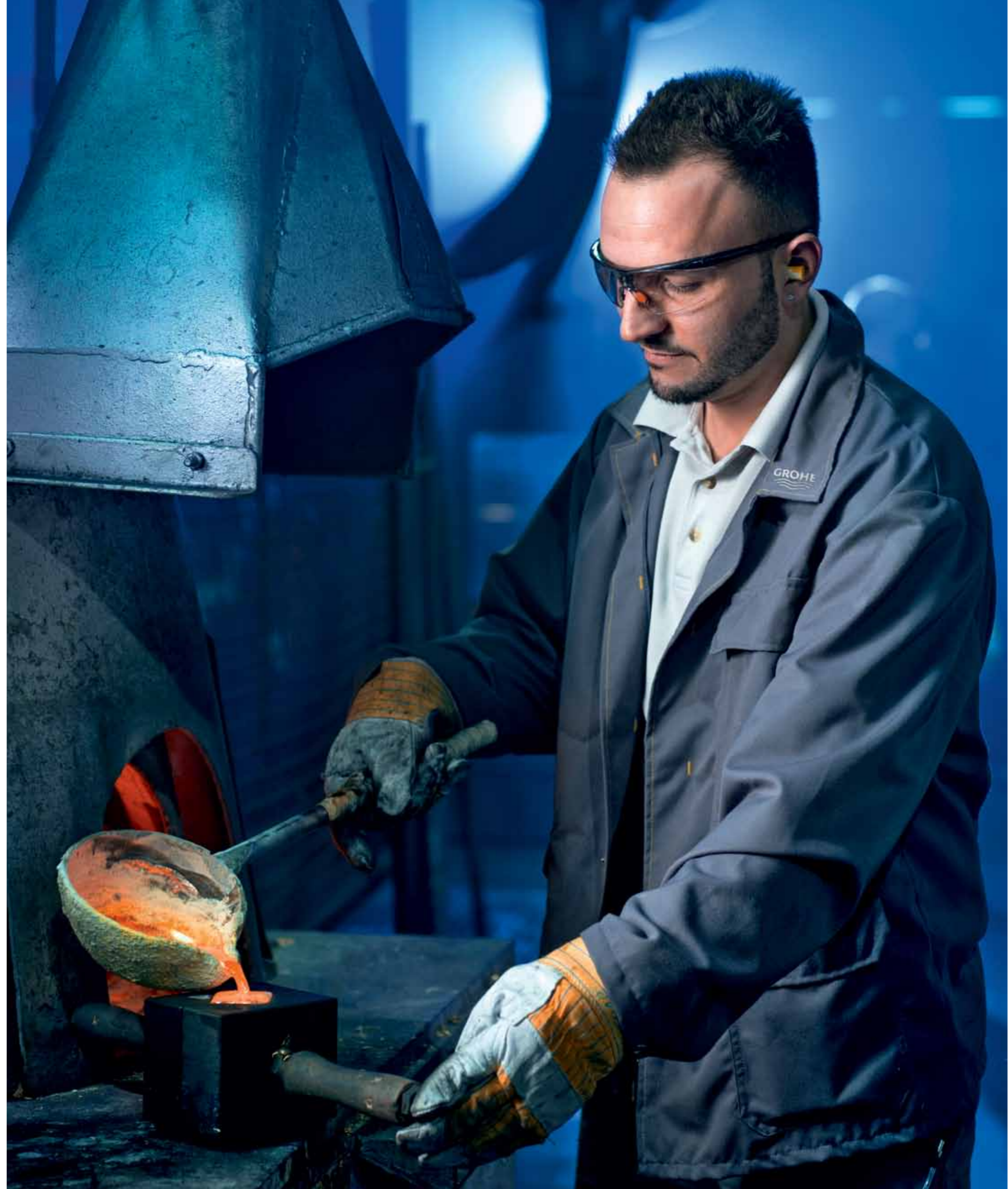
Georgios Vlachodimos, Master of Technology, takes a sample of GROHE's own handmade brass, GROHE Zero®, that ensures our faucets are virtually lead-free and its composition has been proven to be more resistant to corrosion.
