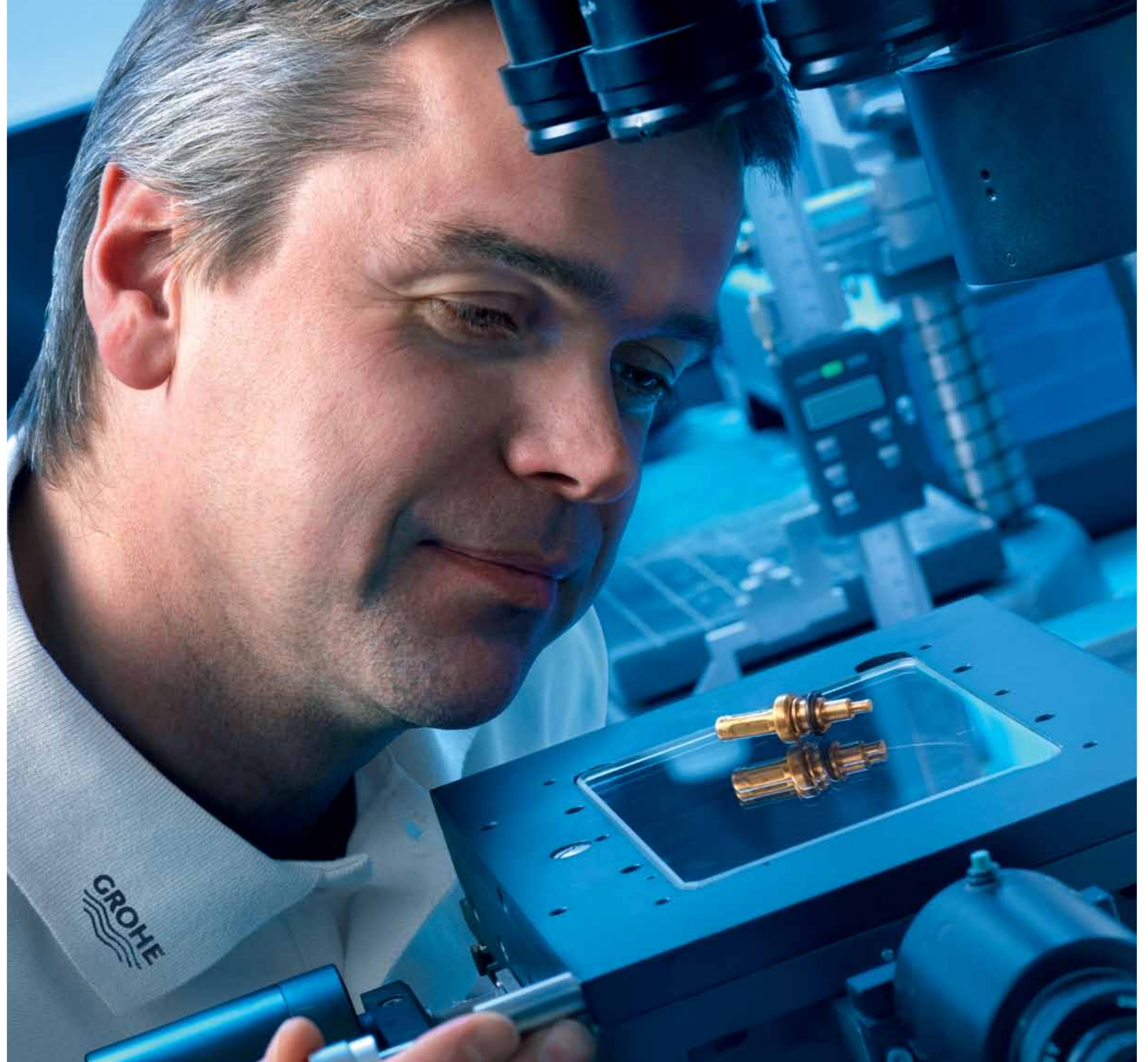
Martin Weiss, Master of Technology, tests the thermocouple in the GROHE TurboStat® cartridge that reacts to changes in water pressure on hot and cold supplies to maintain a constant temperature and flow in the blink of any eye.
