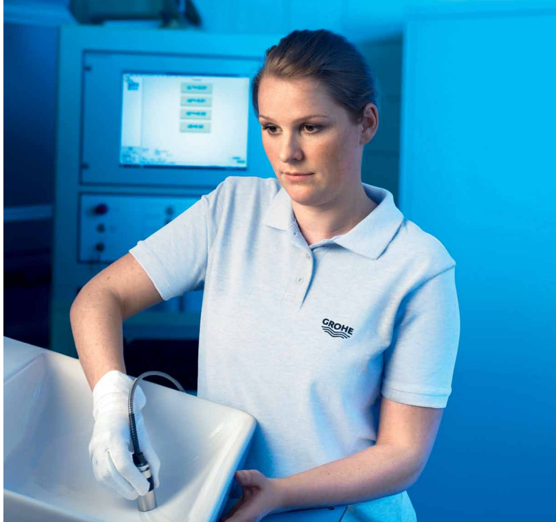
Janika Taschies, Master of Technology, uses a spectrometer to check that the test sample matches perfectly to the ceramic coated with GROHE Hygiene.
