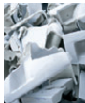
100% recyclable product Sanitary ware is 100% recyclable; granulated material can be returned to the manufacturing process, or it can be employed in other fields of industry.
