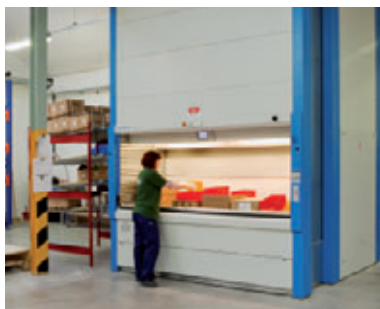
Kardex. Automated high-capacity storage system.
