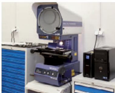
Profile projector. Quality management laboratory.
