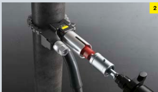
2 Drill using the drill shaft and a conventional drill, then remove the holding device.
