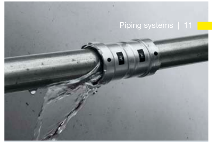
Like all Viega press systems, Megapress also has the tried-and-tested Viega SC-Contur that immediately highlights any inadvertently unpressed connections.
