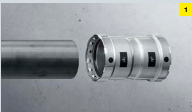
Cut steel pipe to length and clean, mark insertion depth and fit connector up to the marking on the pipe.
